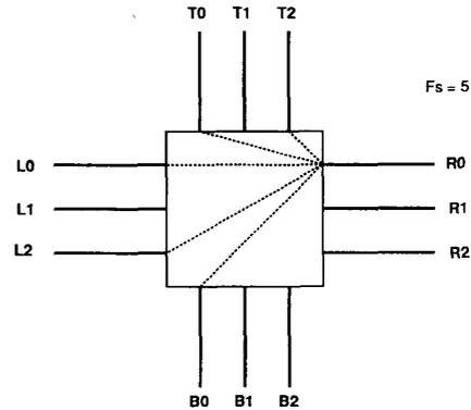
Fig. 2. Definition of flexibility of switch block.
