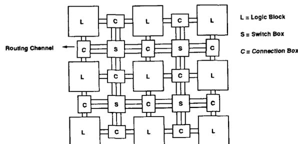
Fig. 1. General routing structure of an FPGA.
