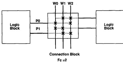
Fig. 4. Definition of flexibility of connection block.
