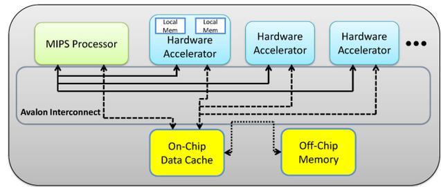
Figure 2. Default LegUp system architecture.
