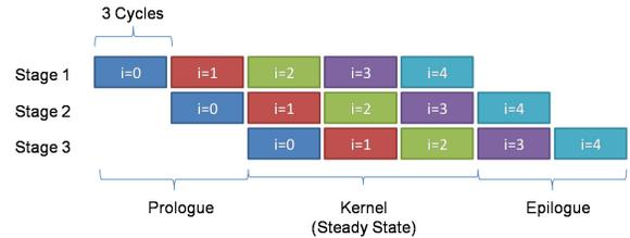
**Figure 5.** Time sequence of a loop pipeline with  $II=3$  and five loop iterations.
