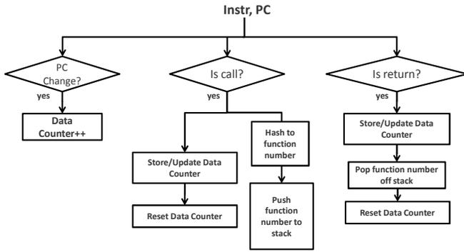
Figure 3. High-level flow chart for instruction-count profiling.
