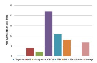
Fig. 6: Area overhead for implementation of input-checking functionality on hardware accelerators with reduced bitwidths.
