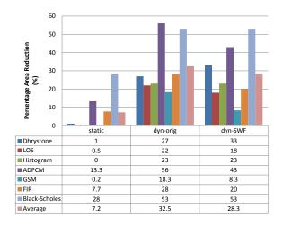
Fig. 5: Percentage area reduction of hardware accelerator synthesized with static and dynamic analysis.
