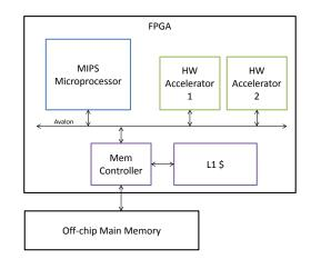
Fig. 1: Hybrid processor/accelerator architecture on FPGA.
