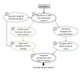
Fig. 2: Hybrid design flow for HLS of hardware accelerators with software fallback.
