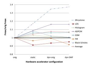
Fig. 9: Increase in maximum accelerator operating frequency for *static*, *dyn-orig* and *dyn-SWF* configurations compared to *orig*.
