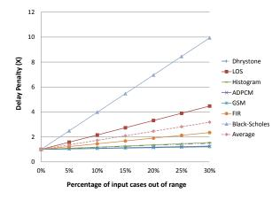
Fig. 8: Software fallback delay increase penalty in relation to the percentage of out of range input datasets.
